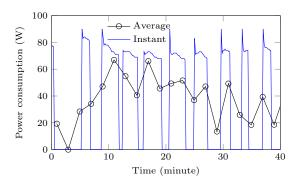
Figure 15: The real-time freezer power consumption (sampled at 10 s) and the average on a 2 minute interval during a portion of the MPC-C experiment.
