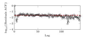
Figure 6: The autocorrelation of Model B residuals (full line) and white noise (dashed line).
