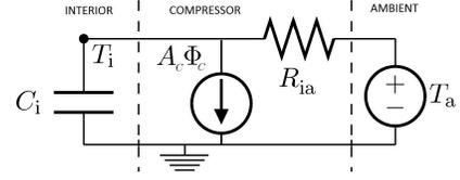
Fig. 2. Refrigerator preliminary model (electrical equivalent):  $T_i$ .
