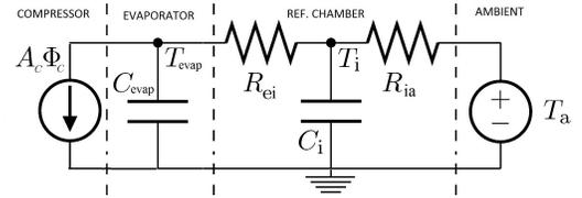
Fig. 3. Refrigerator model (electrical equivalent):  $T_i T_{evap}$ .
