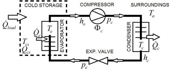
Fig. 1. Single stage vapor-compression refrigeration system.
