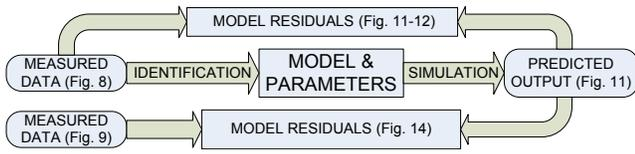
Fig. 6. Process of parameters identification and model validation.
