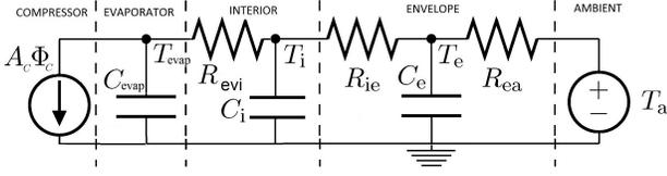
Fig. 4. Refrigerator model (electrical equivalent):  $T_i T_{evap} T_e$ .
