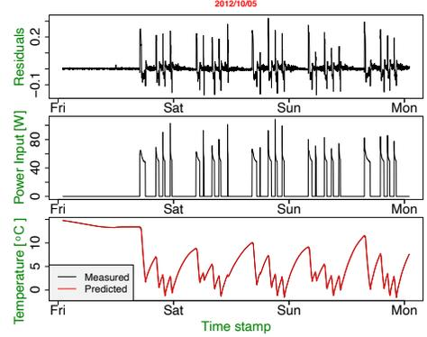
Fig. 10. Residuals, input and output of Model:  $T_i$ .
