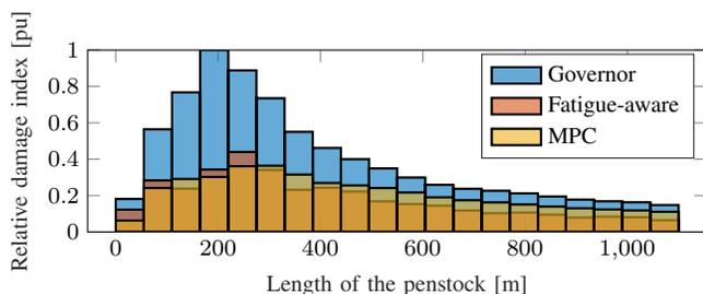
Fig. 8: RDI along the penstock with reference to the case without filtering after fatigue-aware filter and MPC action
