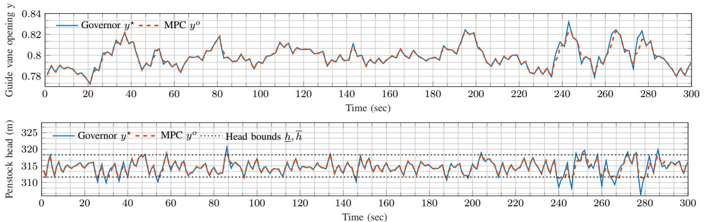
Fig. 5: Set-point actuated by the governor and MPC (top panel) and respective head in the critical portion of the penstock (bottom panel).
