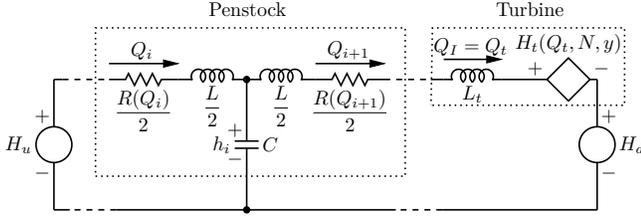
Fig. 2: Equivalent circuit model of a medium-head HPP.
