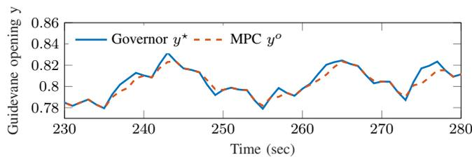
Fig. 6: MPC actuated guide vane set point
