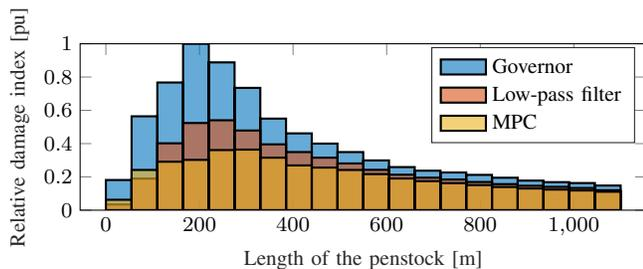
Fig. 7: RDI along the penstock with reference to the case without filtering after low-pass filter and MPC action
