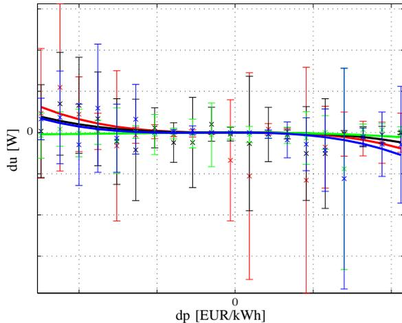
Fig. 7. The price responsiveness for the four different algorithms, defined as the variation in the power consumption as a function of a variation in the price; vertical bars show the standard deviations for the different responses.
