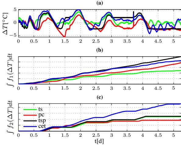
Fig. 5. Plot *a* shows the temperature deviation from the set-point ( $23^\circ\text{C}$ ) for the different algorithms. Plot *b* is the accumulated error (with states of under temperature have been weighted 1.2 times more). Plot *c* is the accumulated error for the temperature deviation from the comfort area that is  $23 \pm 3^\circ\text{C}$ .
