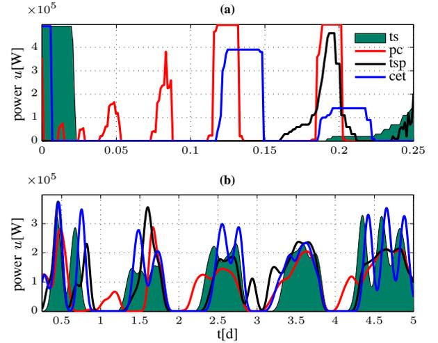
Fig. 4. A comparison of the output of the four different controllers. The two plots are consecutive and with different time scale. Data in the plot *b* have been filtered with a low pass filter for a better visualization of the main frequency components.
