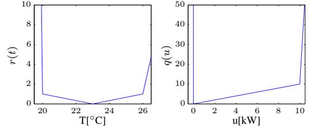
Fig. 2. The weighting functions used in the cost expression of the MPC.
