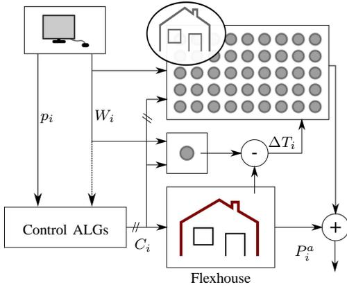
Fig. 1. The experimental setup used for the proposed simulations with the FlexHouse building as the *hardware-in-the-loop* for reproducing the real environmental conditions. Weather forecast  $W_i$  and the price  $p_i$  signal are used.
