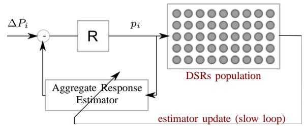
Fig. 1. The proposed control approach. A model is used for predicting the aggregated power response from all DSRs; a closed control loop with a regulator is used for producing the control signal to send to the population of buildings. Subscripts  $i$  refers to the discretized time interval  $t = i$ .
