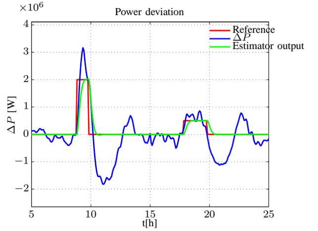
Fig. 4. The blue line shows the response of the aggregated power consumption of DSR units to multiple steps variation of the power reference which is the red line; the green line is response of the estimator.
