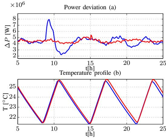
Fig. 3. Plot (a) shows the different profiles of the aggregated power response of the population of demand side resources when they are required to support the grid (blue line) and when not (red line). Plot (b) shows the indoor temperature behavior of one of the building of the population both when its thermostat is controlled by the demand side algorithm and when the set point is the optimal indoor comfort level.
