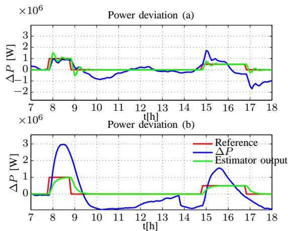
Fig. 5. Power deviation reference, DSRs aggregated power response and estimated power response for two different experiments. Control loop does not perform well in plot (b) because non linearities introduced by the control algorithm and thermostatic cycle starts to emerge because a low number of units is using electric power in the same time.
